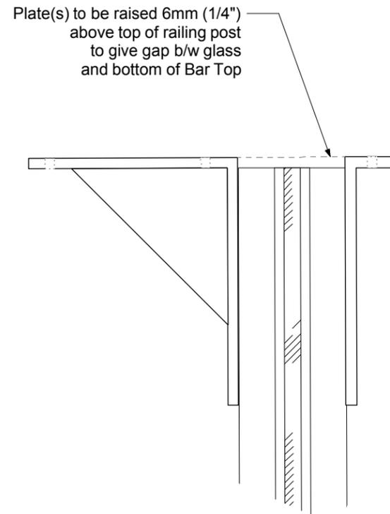
14 Elevation: Bracket to Railing
