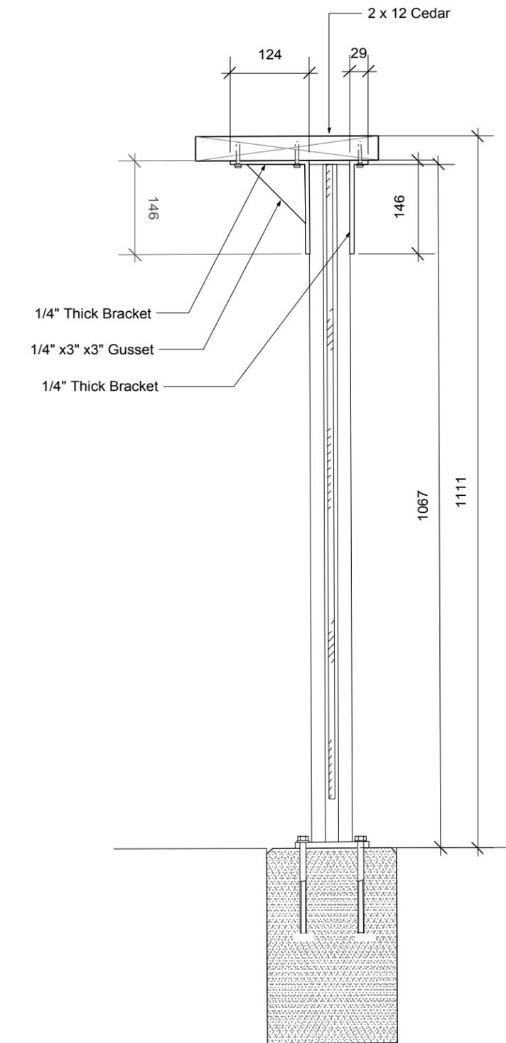
13 Elevation: Railing, Bracket and Bar Top Assembly
